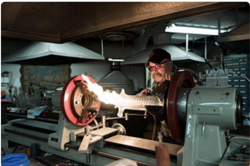
The glass blowing shop handles the fabrication and repair of instructional and research glassware. Stock sizes of glass tubing, rod, ground glass joints, stopcocks, glass-metal seals, etc., are available.
